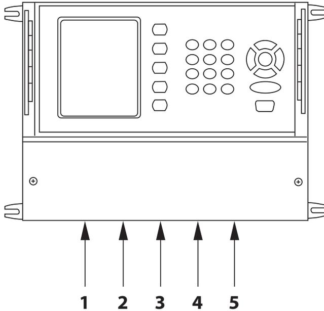
The bottom of the Accuron enclosure is furnished with (5) 1/2" conduit entrances
