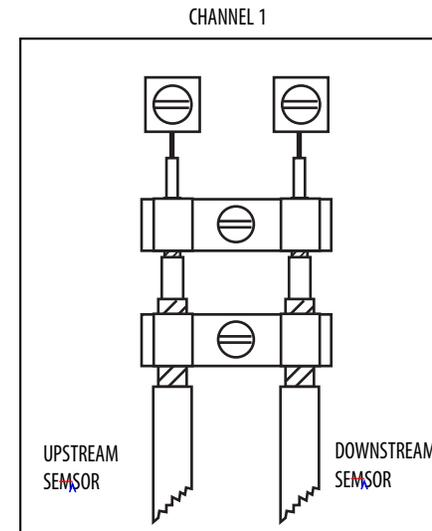
Take the upstream cable and insert the center conductor into the upstream terminal connection and tighten the screw. Slightly pull on the cable to insure the wire is secured to the terminal. Take the downstream cable and insert the center conductor into the downstream terminal connection and tighten the screw. Slightly pull on the cable to insure the wire is secured to the terminal.
