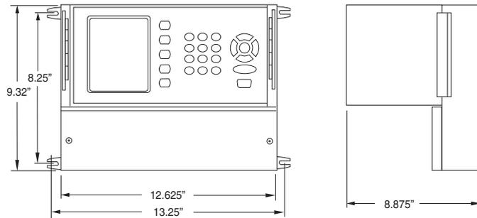
**Do not face the display towards the sun. A sunshade must be used for outdoor installation. Conduit openings must be properly prepared and sealed to maintain the NEMA 4X rating.** The enclosure is rated IP 66 (NEMA 4X) and can be mounted indoors or out. There are two stainless steel mounting brackets attached to the enclosure.
