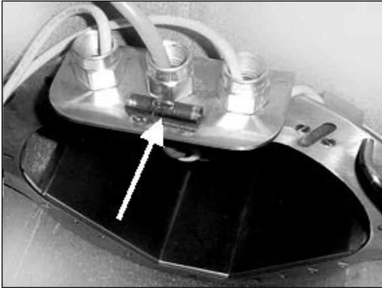
Rotate the Cartridge until the bubble in level provided is centered.
