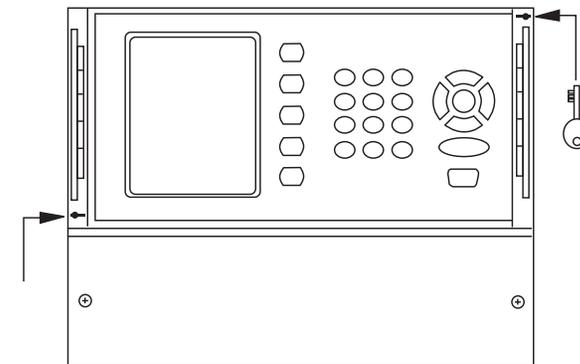
Two plastic gray plugs are supplied with the Accuron meter housing. The plugs may be utilized to permanently lock either side of the cover by inserting them into the keyhole. The optional Keylock may then be used to lock and unlock the other side of the cover. The key can only be removed if the cover is in the locked mode.
