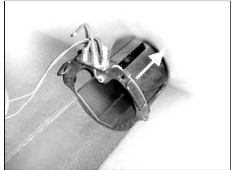
Slide the Cartridge into the pipe until the upstream flange is in contact with the wall.
