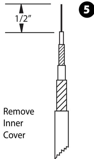
**USE DRAWING BELOW AS TEMPLATE FOR CONFIRMATION OF CORRECT CABLE PREPARATION**
