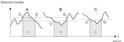
$A = Maximum safety \rightarrow ① SWITCH-OFF POINT > ② SWITCH-ON POINT$
