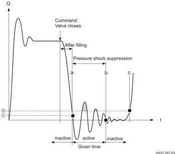
① = switch-on point (for low flow), ② = switch-off point (for low flow)
