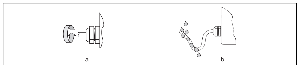
Fig. 40: Installation instructions, cable entries
