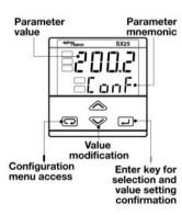
Press or void to display the next parameter or the next code and change its value. The new value entered is stored into the controller when the next parameter is selected by
