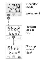
The green led immediate will flash when the Fuzzy Tuning is in operation. At the end of this operation, the calculated PID values are stored and used by the control algorithm and the controller automatically returns to the operator mode. The green led immediate will switch off. The self-learning Adaptive Tuning is non-intrusive. It doesn't affect the process during the calculation of the optimal PID values.
