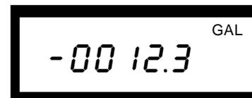
6. Scaled pulse resolution: This screen uses the unit of measure and the six digit display to show the amount of consumption that one scaled output pulse represents. A "P" is used to indicate this screen. The example below represents one pulse as equaling ten gallons.
