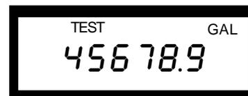
5. Backflow: This screen is identical to totalization except it is only 5 digits preceded by a negative sign. The negative sign indicates the backflow screen. The resolution of the backflow screen is the same as in the test mode. The backflow screen shows the total amount of reverse flow through the meter.
