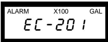
When an alarm occurs an error code displayed. The key for each alarm is the first number after the EC. Error codes are listed below. The XX represents other internal programming numbers.
