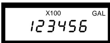
2. Rate of Flow: Rate is shown as a 5 digit display without a multiplier. The unit of measure (GAL, FT3, M3, IMP, LITER) will be shown with the corresponding time unit (per MIN, per HOUR). The flow rate resolution will vary with meter size. There are no multipliers used for flow rate. Flow in the reverse direction is displayed with a negative sign.
