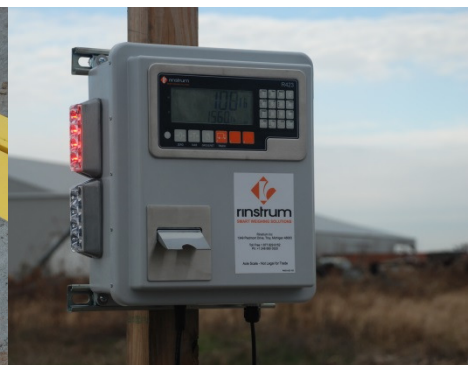
Step 9: Install controller and complete electrical connections. Apply power and weigh trucks
