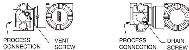
Figure 19. Horizontal Mounting - Cavity Venting and Draining
