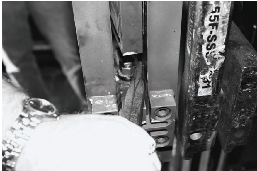
Figure 2-14. Centering the Load Cell Using a Chisel
