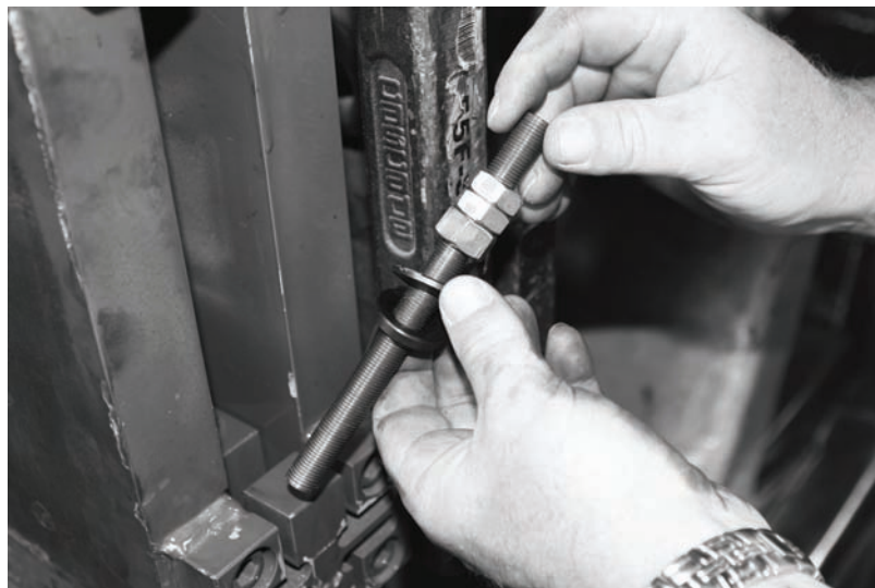
Figure 2-12. Install Spherical Washer Set
