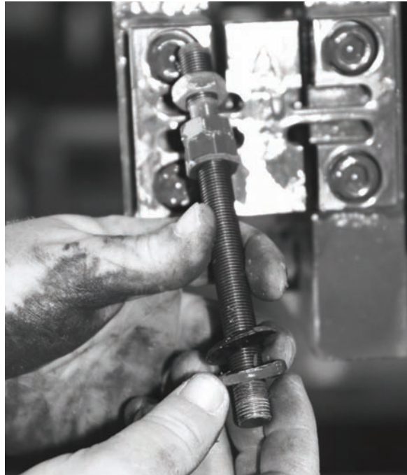
Figure 2-7. Remove Flexure Rod with Nuts and Washers
