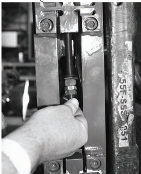
Figure 2-10. Installing Flexure into Scale
