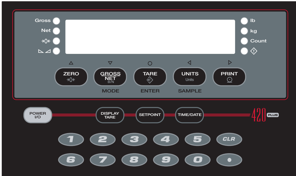
Figure 1-1. 420 Plus Front Panel, Showing LED Annunciators and Normal Mode Key Functions
