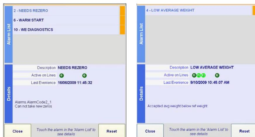
Figure 2-9. Alarm Panel—Multi-Line
